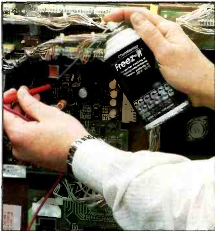
Figure 4. Alternately heating and cooling suspected components can help to pinpoint the cause of failure. (Photo courtesy of Chemtronics)
